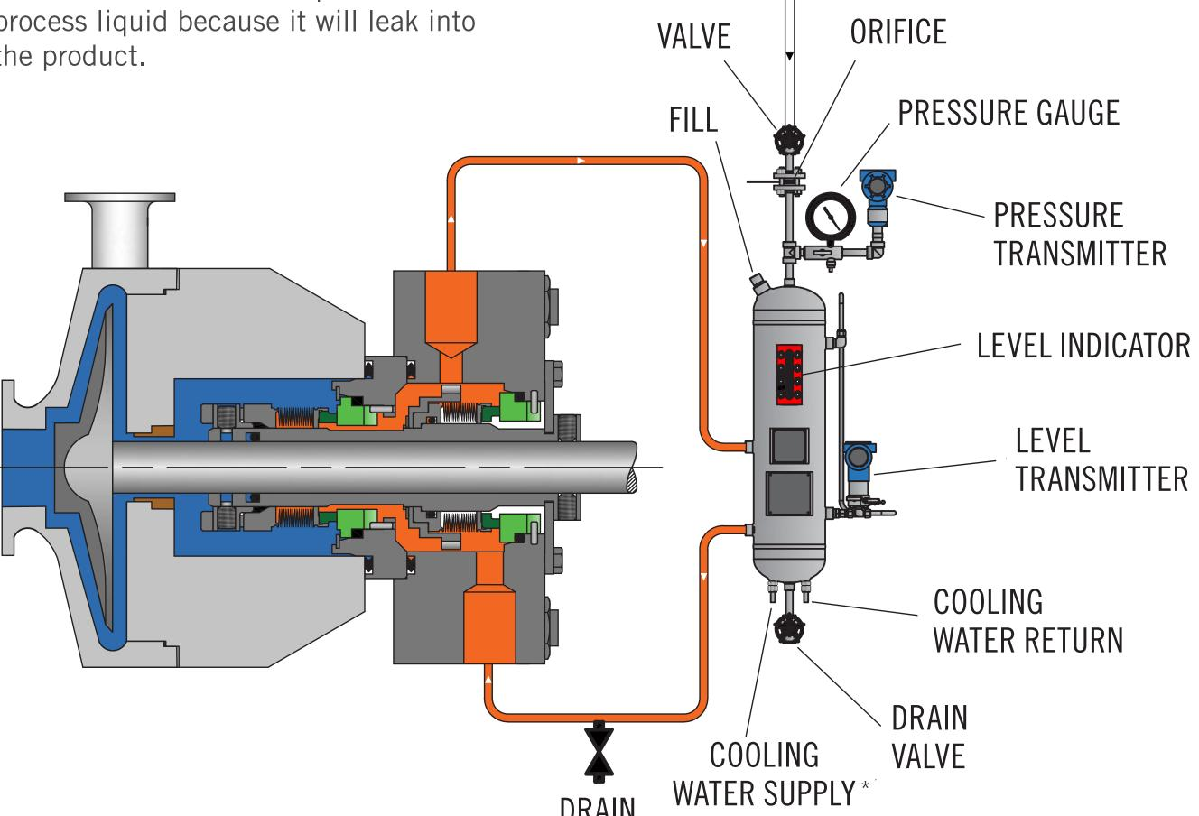
NOTE: Continuous pressurization with nitrogen, not air, is recommended. Generally for barrier pressures above 150 psi (10.3 bar) use Plan 53B, 53C or 54. Consult Flexaseal for best practices in all applications.
