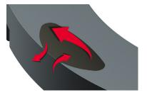
**Ultra-Polished Dynamic O-Ring Surfaces** and backup ring design minimize O-ring parasitic drag for a fast seal response to changing conditions
